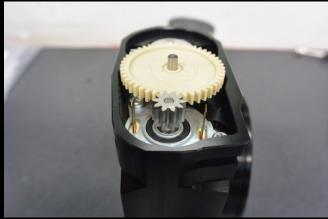
6. Reinstall the factory cover, make sure the oring stays in place during assembly and the (2) electrical connections are made.
