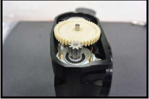
2. Remove the (6) throttle body cover tabs by releasing using a small pick or screw driver.
