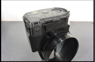
7. Reuse the (6) throttle body cover tabs by pressing on until they click and lock in place.
